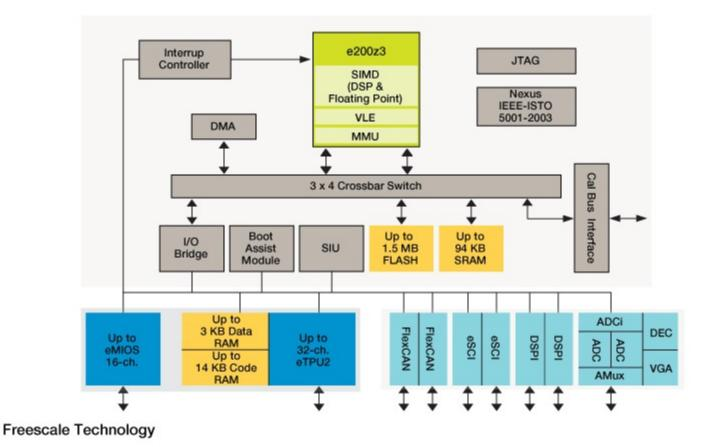
32 BIT 80 Mhz 80 GPIO AD/DA CAN FLASH SYSTEM ON CHIP 1181 PAGE REFERENCE MANUAL 4 CYLINDER VERSION
